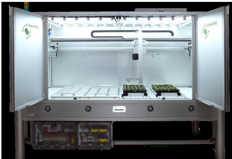
Figure 2: ScanalyzerHTS developed by LemnaTec [3] to study plant phenotyping in simulated environments
